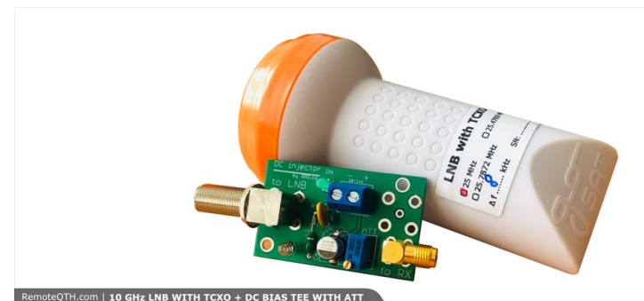
RemoteQTH.com | 10 GHz LNB WITH TCXO + DC BIAS TEE WITH ATT
